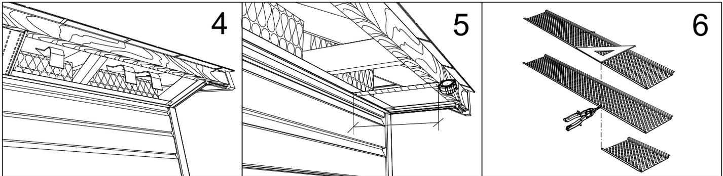
4 Verify that there is sufficient air space between the insulation and underside of the roof deck, correct if necessary. Verify that the insulation is in good condition and that it has been properly installed.
