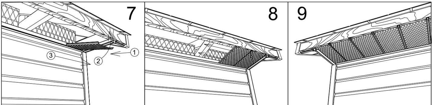
7 Slide the soffit onto the existing J-Trim, making sure that the soffit is all the way in and laying completely flat on the trim. Make sure it is straight and flush with the fascia board. Refer to the steps shown above.
