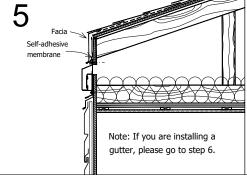
Install a self-adhesive membrane over the edge of the Anti-Gust Wall Soffit. Re-install or install a facia and/or the exterior siding over the soffit.
