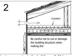
Create an opening in the building wall. Make sure that this opening is over the attic insulation. This opening should equal to the dimension of the soffit ordered. (either 1.25" or 1.75" depending on the model)
