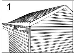
On an existing building, remove a section of exterior siding at the chosen installation location. If you are installing on a new building, please skip to step 2.
