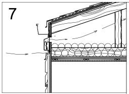
Air circulation through the Anti-Gust Wall Soffit .
