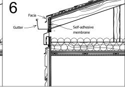
For the gutter installation (if needed), install a self-adhesive membrane over the top edge of the soffit to prevent a direct contact between the gutter and the soffit. Complete the installation of the gutter and the facia as shown.
