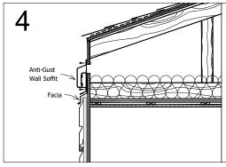
Place a facia over the exterior siding and attach the Anti-Gust Wall Soffit over it using screws or nails at the location shown. (coordonate this installation depending on the installation location and exterior siding)
