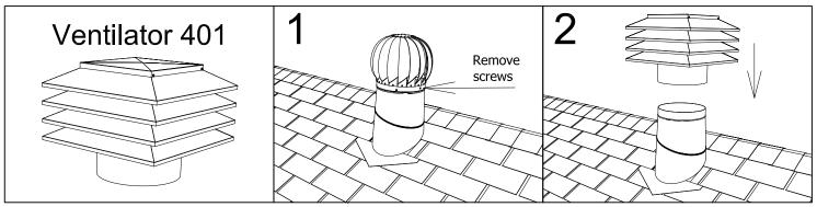
Remove the screws that are securing the turbine head onto the base flashing. Verify that the base is in good and solid condition as well as the sealant to prevent any rain or snow infiltrations.
