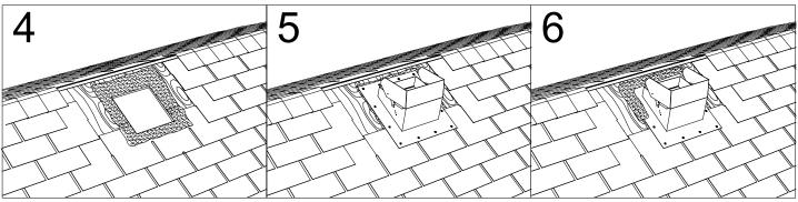
apply a generous amount of bitumen cement over the top portion of the shingle parallel with the hole as illustrated.
