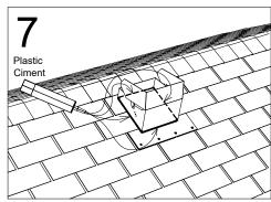
Re-install shingles around flashing and deck complete. Finish by applying a sealant around the base on all four sides.
