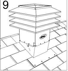
Install ventilator head onto the flashing, making sure it is level and that all louvers are above the ridge and secure to the flashing using screws provided into each of the perforations. Please make sure that the bottom deflector of the ventilator is standing 6in above the ridge line. (Model 301 shown)
