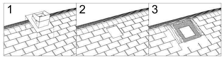
Place flashing over desired area making sure it is positioned between the rafters, and trace a line onto the shingles using the inside duct as a template. Opening should start 6-8 inches down from the ridge.
