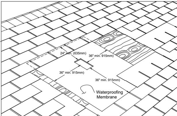
**Existing Roof:** Remove the shingles around the opening dedicated to the installation of the roof exhaust in order to install a waterproofing membrane around the hole as shown above.
