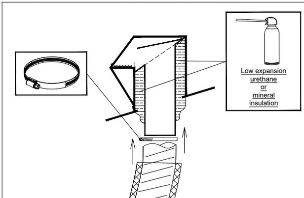
Install mineral-type insulation or low expansion urethane type insulation between the flap walls and the exhaust duct. Make sure to install insulation tightly all around the exhaust duct without leaving any empty spaces. Install an insulated flexible duct (2" insulation recommended) on the roof exhaust duct using an adjustable collar. Seal tightly with duct tape.
