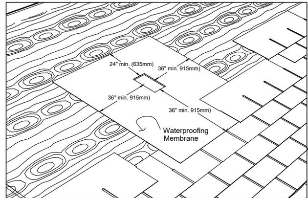
**New roof:** Install a waterproofing membrane around the opening dedicated to the installation of the roof exhaust as shown above.
