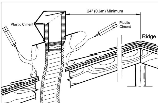
Apply plastic cement generously around the perimeter of the opening making sure to maintain a width of 4 inches. Slide the flexible duct into the opening, followed by the roof exhaust unit making sure the flashing is fully embedded in the plastic cement. Nail or screw the unit to the bridging (1 inch from the edge of the unit) while leaving a spacing of 4 inches. Finish by applying a generous amount of plastic cement to the back and sides of the flashing.
