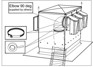
Remove the top cover of the CTM and install a 90deg elbow of the right size over the collar of the AF traps, using an adjustable collar. Secondly, install a duct (flexible 2in insulated duct is recommendeded) around the 90 deg. elbow using an adjustable collar. Seal all connections using a good quality duct tape.
