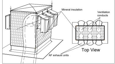
Fill-in the remaining space around the duct with mineral insulation and re-install the cover of the CTM-MB, making sure of tightening all screws.
