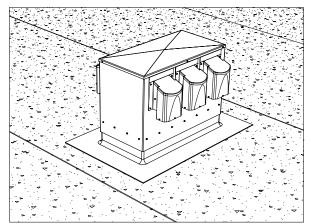
Install the head of the CTM on its flashing by fastening it to the flashing using the supplied self-tapping screws. Make sure to install the screws at a minimum height of 203mm (8') from the finished roof system.
