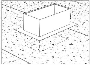
Place the flashing on the roof at the desired location. Make sure the opening is located between the structural beams. Trace a line on the roof from inside the curb.
