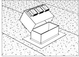
Place the head of the CTM over its flashing.
