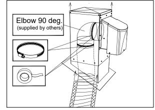
Remove the top cover of the CT-AD-12 and install an 90deg elbow of the right size over the collar of the AF trap, using an adjustable collar. Secondly, install a duct (flexible 2in insulated duct is recommendeded) around the 90 deg. elbow using an adjustable collar. Seal all connections using a good quality duct tape.
