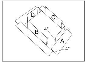
A galvanized metal counter flashing (4" high x 4" flange) as illustrated above will need to be installed, this item is sold separately.
