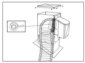
Fold the polythene (vapor barrier) over the insulation and push it to the bottom of the roof exhaust unit to ensure that the entire duct is covered. Finish by fixing it with a good quality duct tape. Ensure there are no exposed or uninsulated duct sections.
