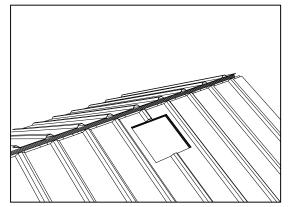
Locate where the roof exhaust/inlet unit will be located and cut out an opening in the roof deck to reflect the same size opening of the sloped flashing to be installed.
