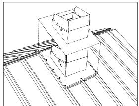
Install slope flashing over the counter flashing and fasten onto metal roof and deck (screws supplied by contractor). Install a quality bitumen sealant around the perimeter of the flashing, filling up all gaps between metal and flashing. 6
