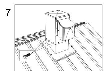
Install CT-AD-12 head onto the flashing, making sure it is level and secure to the flashing using screws provided into each of the perforations.
