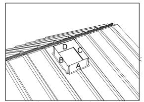
Remove a few screws and lift metal roof, slide counter flashing parts (A, B, C, and D) between wood and metal components. Re-install srews and seal all joints with bitumen tape or caulking.
