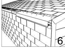
Install the first length of mansard soffit making sure you follow the traced line and secure to deck with screws (screws supplied by contractor).
