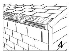
Re-install 1 row of shingles on the mansard roof, then cut out the surplus that is covering the opening as per illustration.
