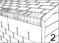
Remove drip edge and last two rows of shingles on the mansard. Trace a line starting from the top portion of the mansard down 2.5 inches straight across as per illustration
