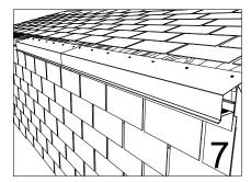
Install a second length overlapping the first by 2 inches and secure to deck, again making sure you follow the traced line. Repeat step #7 for all that follow as per illustration.
