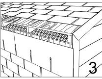
Cut out opening in mansard deck by following the line, exposing the rafters and insulation as per illustration. Be careful not to cut or interfere with the rafters. Make sure that the insulation will not be obstructing air flow into the attic.
