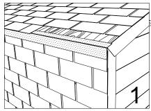
Start by removing the first two rows of shingles on the slope roof exposing the deck at the juncture as per illustration
