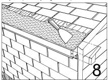
Install the end caps onto each extremity and secure with screws provided. Apply a bitumen sealant over the flashing complete as per illustration.
