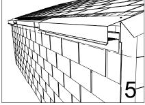
Temporarily install 2 lenghts of the mansard soffit drip edge, one at each extremity and make sure that the bottom flashing is tight against the mansard roof and shingles, then trace a line onto the roof deck making sure that they are perfectly aligned as per illustration.
