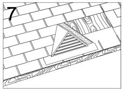
Re-install shingles around flashing and deck complete as per illustration.
