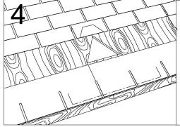
Carefully remove the shingles around the perimeter of the hole to expose deck as per illustration.
