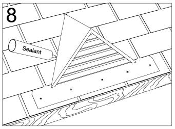
Secure bottom flange using galvanized roofing screws with rubber rings. Finish by installing a bead of sealant around perimeter of unit, sealing all joints.
