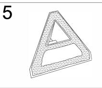
Apply a generous amount of bitumen sealant onto the underside of the flashing, secure to deck with screws. (screws supplied by contractor)
