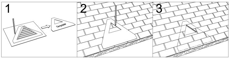
Using cardboard or other thin material, make a template of the underside of the unit including the opening.
