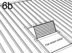
**Existing roof:** Slide the AT1 under the adjacent roof steel panels (3 sides) and center over the opening already cut. Place a flat sheet metal panel at the bottom and under the flashing of the AT1 up to the edge of the roof.
