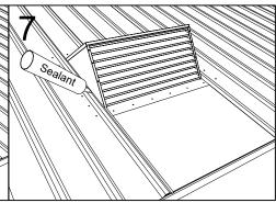
Secure bottom flange using galvanized roofing screws with rubber rings on the 4 sides of the AT1 (supplied by contractor). Finish by installing a bead of sealant around perimeter of unit, sealing all joints.
