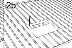
**Existing roof:** Place template, making sure the opening is positioned between the rafters, at a few feet from the edge of the roof and over the insulation. Trace and cut an opening in the center of the template.
