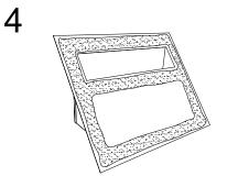
Apply a generous amount of bitumen sealant onto the underside of the flashing.
