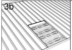
**Existing roof:** Remove the steel roof panels from the opening up to the edge of the roof.
