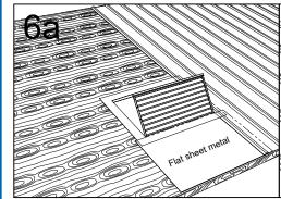
**New roof:** Slide the AT1 under the roof steel panels and center over the opening already cut. Place a flat sheet metal panel at the bottom and under the flashing of the AT1 up to the edge of the roof. Finish the roof installation.
