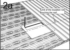
**New roof:** Place template, making sure the opening is positioned between the rafters, at a few feet from the edge of the roof and over the insulation. Trace and cut an opening in the center of the template.
