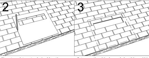
Place template onto desired location, making sure the hole is positioned between the traced line of the hole. the rafters, then trace a line around the perimeter of the template as well as the hole using a chalk.
