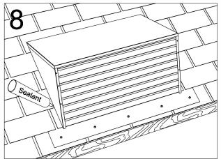
Secure bottom flange using galvanized roofing screws with rubber rings. Finish by installing a bead of sealant around perimeter of unit, sealing all joints.
