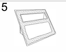
Apply a generous amount of bitumen sealant onto the underside of the flashing, secure to deck with screws. (screws supplied by contractor)
