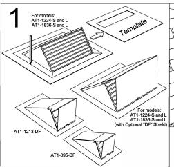
Using cardboard or other thin material, make a template of the underside of the unit including the opening.
