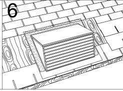
Apply a generous amount of bitumen sealant onto top of flashing as per illustration.
