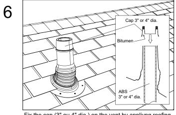
Fix the cap (3" ou 4" dia.) on the vent by applying roofing cement on the inside of the cap, on the top edge of the vent and the ABS pipe. Make sure that you press down the cap outside the vent and inside the ABS pipe.
