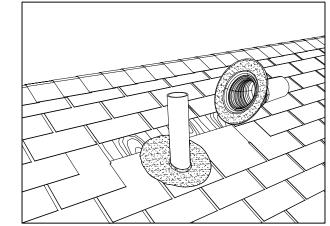
Following the ABS vent pipe installation by the plumbing contractor, carefully remove shingles around the perimeter of the hole to expose the deck and the lower shingles, then apply a generous amount of roofing cement around the perimeter of the hole and under the flashing of the vent.
