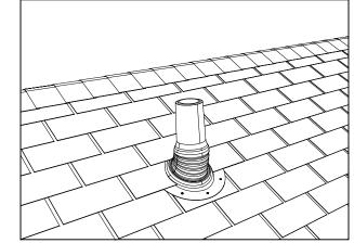
Cut and carefully re-install the shingles removed at step 3.
