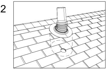
Upon locating the plumbing vent in the attic space, trace and cut a hole at the desired location and to the pipe size diameter. The opening may be located anywhere on the roof deck.
