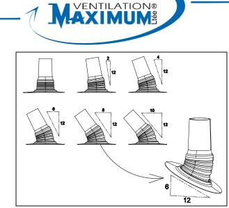
Using the bending tool, form the vent according to the slope of the roof, before installation (from flat roof to a slope of 10/12).
