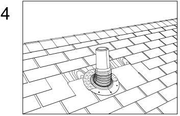
Install the vent over the opening and onto the roofing cement, securing it to the deck. (screws supplied by other) . Apply roofing cement on the top portion of the flashing and halfway down each side.
