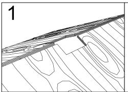
Cut out opening in roof deck to reflect the same size opening of the ridge flashing to be installed.
