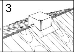
Assemble and fasten the counter flashing onto roof deck around the perimeter of the opening.
