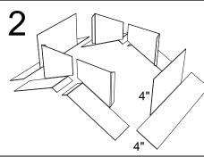
Fabricate a galvanized metal counter flashing (4" high x 4" flange) as illustrated above, supplied by contractor.
