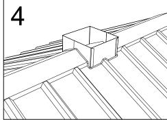
Install metal roof & ridge cap over the counter flashing as illustrated above and then seal around all joints with bitumen tape or caulking.
