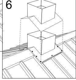
Install ridge flashing over the counter flashing and fasten onto metal roof and deck (screws supplied by contractor). Install a quality bitumen sealant around the perimeter of the flashing, filling up all gaps between metal and flashing.
