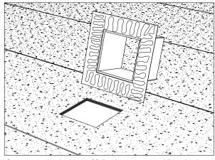
Cut an opening in the roof following your traced line. Apply a generous amount of bitumen under and along the perimeter of the insulated flashing.
