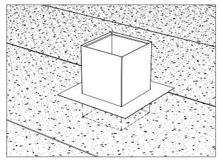
Place the flashing on the roof at the desired location. Make sure the opening is located between the structural beams. Draw a line on the roof from inside the flashing.
