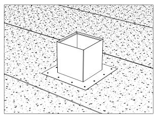
Install the flashing centered on the opening and fasten it to the roof using screws. (fasteners supplied by the contractor) 4
