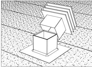
Place the head of the ventilator over its flashing
