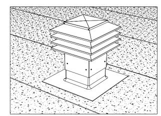
Install the head of the ventilator on its flashing by fastening it using the supplied self-tapping screws. Make sure to install the screws at a minimum height of 203mm (8') from the finished roof system.
