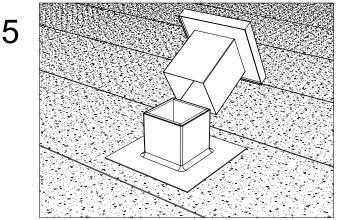
Place the head of the ventilator over its flashing.
