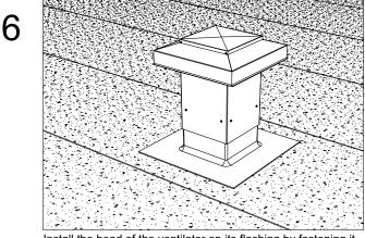
Install the head of the ventilator on its flashing by fastening it to the flashing using the supplied self-tapping screws. Make sure to install the screws at a minimum height of 203mm (8') from the finished roof system.
