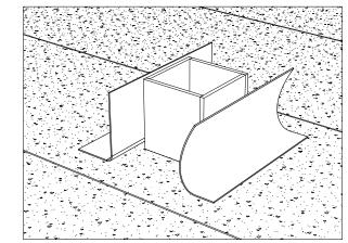
Waterproof the flashing by installing a membrane on all its horizontal and vertical surfaces. Follow the installation instructions recommended by the membrane manufacturer.
