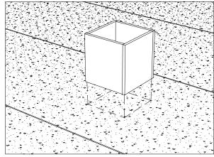
Build a wooden curb to fit inside the vent with the proper allowance for the membrane and place the curb on the roof at the desired location. Make sure the opening is located between the structural beams. Trace a line on the roof from inside the curb.
