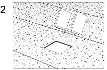
Cut an opening in the roof following your traced line. Apply an amount of bitumen under and along the perimeter of the curb.
