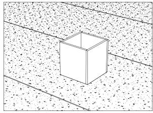
Install the curb centered on the opening and fasten it to the roof using screws. (fasteners supplied by the contractor)
