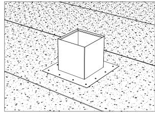
Install the flashing centered on the opening and fasten it to the roof using screws. (fasteners supplied by the contractor)
