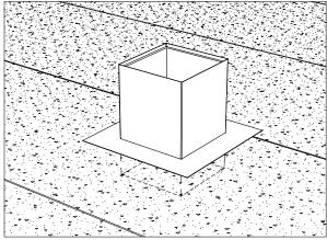
Place the flashing on the roof at the desired location. Make sure the opening is located between the structural beams. Trace a line on the roof from inside the flashing.
