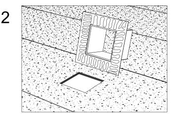
Cut an opening in the roof following your traced line. Apply a generous amount of bitumen under and along the perimeter of the insulated flashing.
