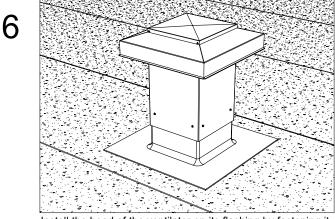
Install the head of the ventilator on its flashing by fastening it using the supplied self-tapping screws. Make sure to install the screws at a minimum height of 203mm (8') from the finished roof system.
