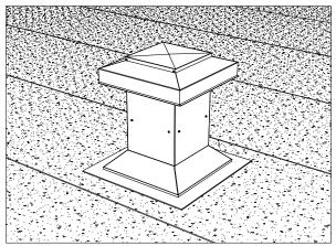
Install the head of the ventilator on its flashing by fastening it to the flashing using the supplied self-tapping screws. Make sure to install the screws at a minimum height of 203mm (8') from the finished roof system.
