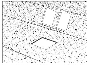
Cut an opening in the roof following your traced line. Apply an amount of bitumen under and along the perimeter of the curb.
