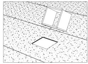
Cut an opening in the roof following your traced line. Apply a generous amount of bitumen under and along the perimeter of the curb.
